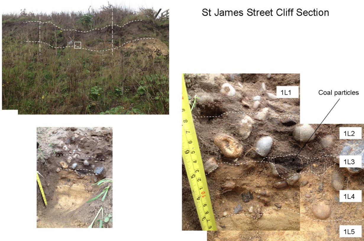
Figure 6: St James Street cliff section showing context (left) and detail of the bottom sediment section including stratigraphic layers (details in Appendix 3.0). Location of coal deposit is shown which precluded radiocarbon dating. Section 1L5 is in-situ cliff material.
