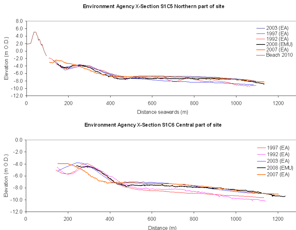
Figure 43 Bathymetric changes across the northern and middle sections of the Dunwich town site. The largest changes occur where morphological change occurs such as the migration of the inner sand bank between 200-400m from datum.
