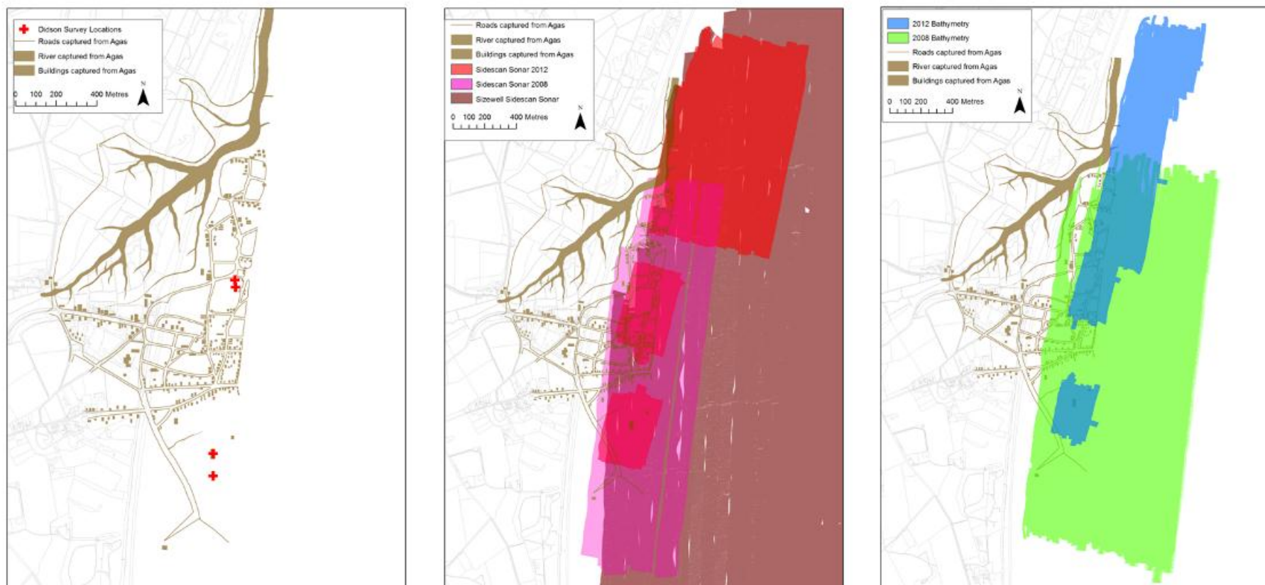
Figure 8 Survey areas for available geophysical data. Left; DIDSON acoustic imaging; Centre – Sidescan Sonar data, Right Multibeam data.
