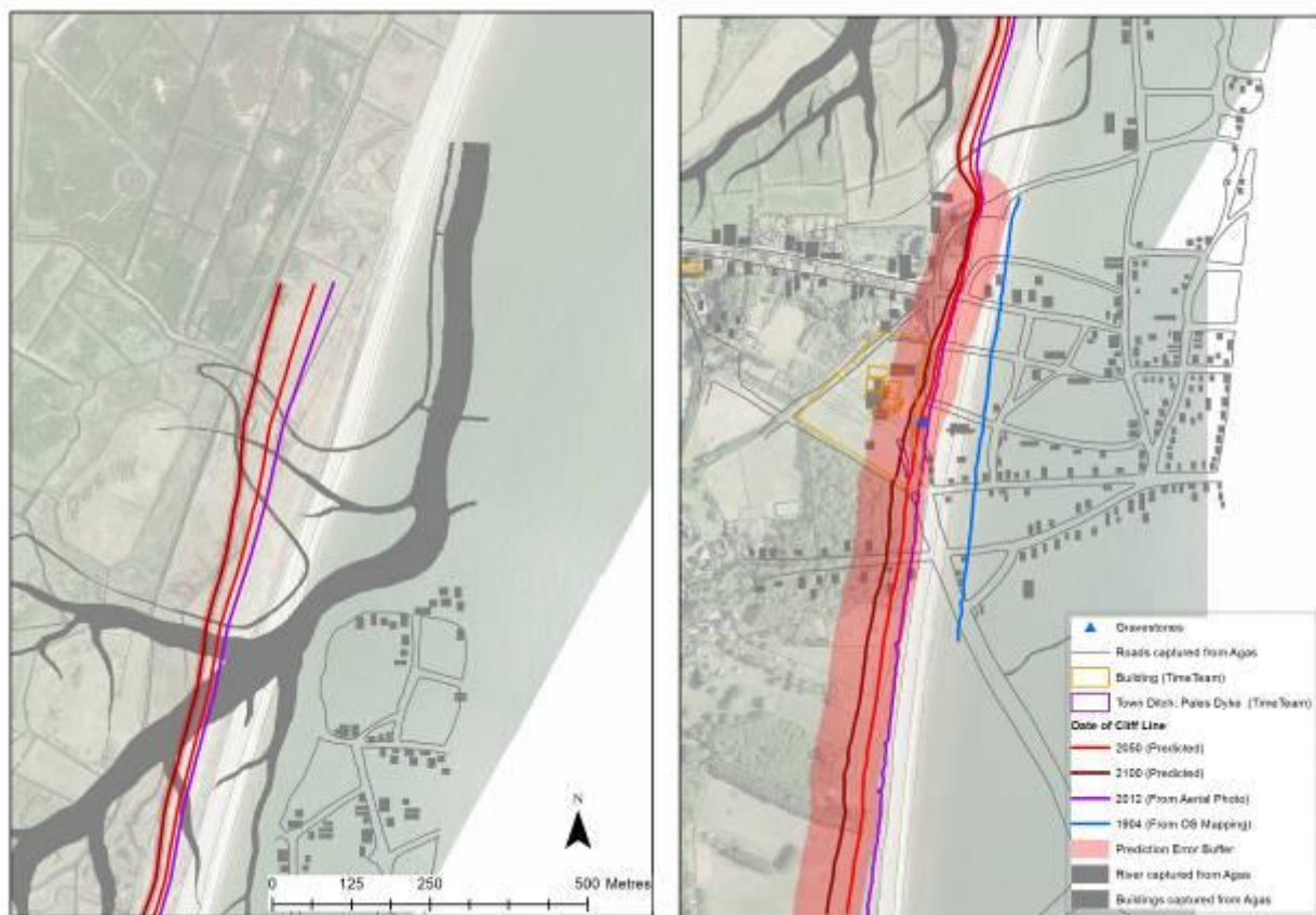
Figure 49 Future coastlines forecast using linear extrapolation of cliff positions 1904-2012. Buffer is based on RMSE for forecasts vs observed coastal positions. Archaeology at risk is summarised in Table 9.
